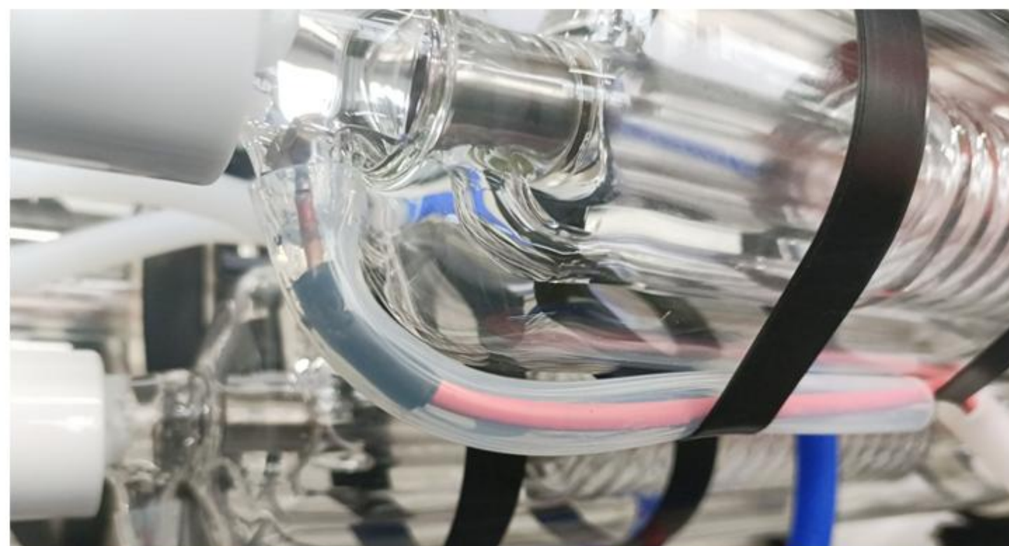
High-Voltage Wire Insulation
