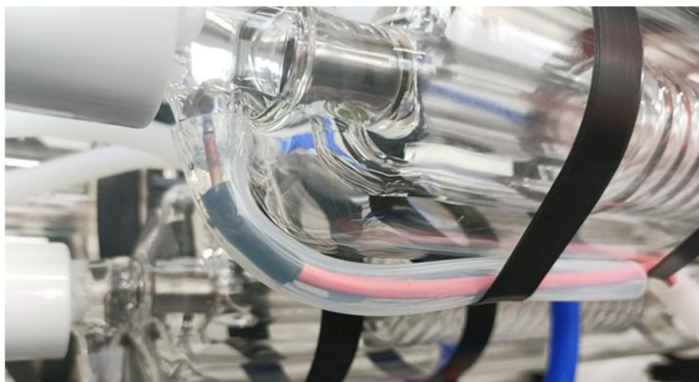
High-Voltage Wire Insulation
